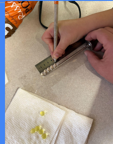
Measuring wet beads. Photo by C.Provencio
