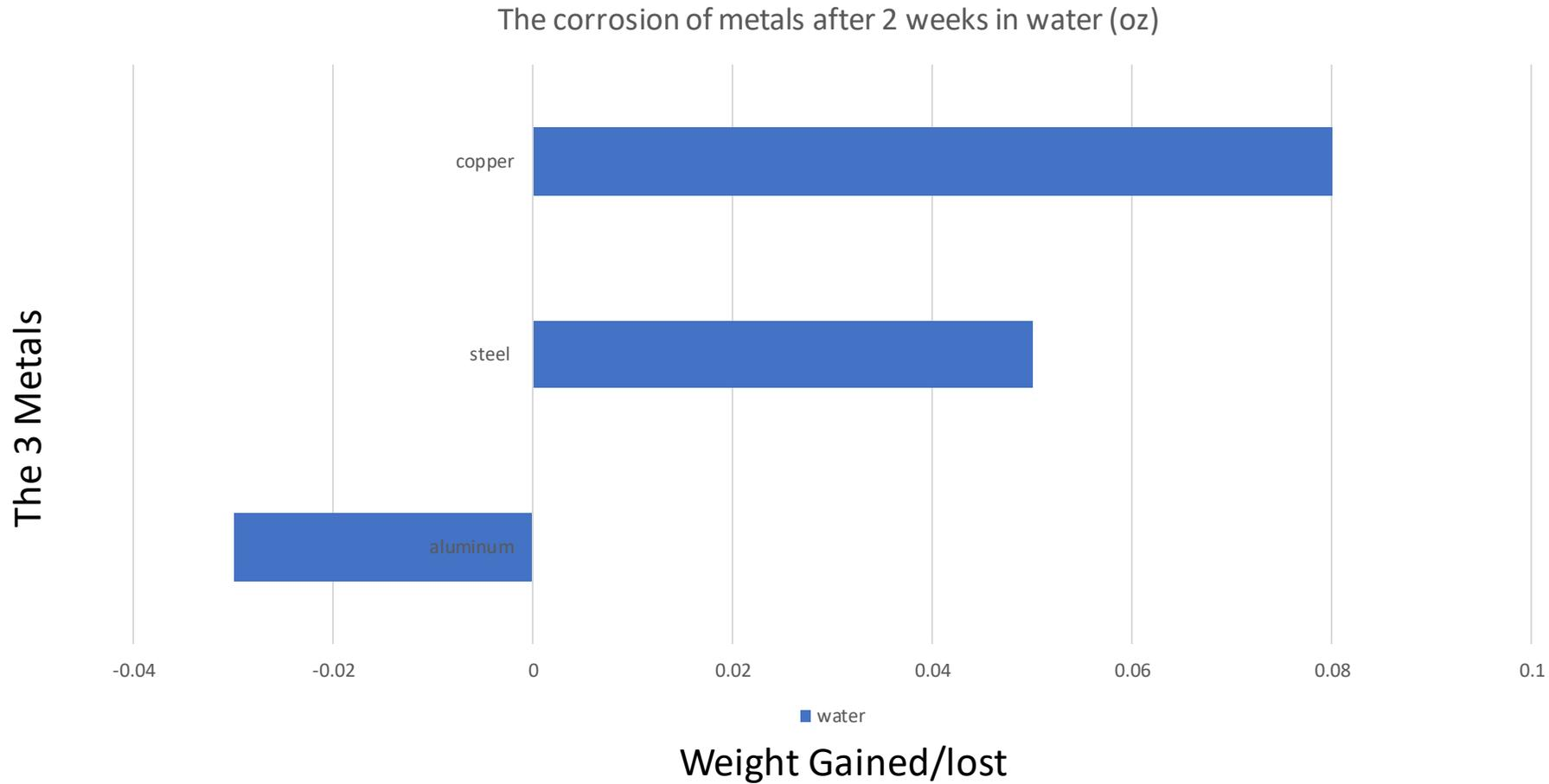
The bar graph will show in a visual form the difference of in weight of the metal in how much it gained or lost (in oz) due to Oxidation/Hydroxylation.
