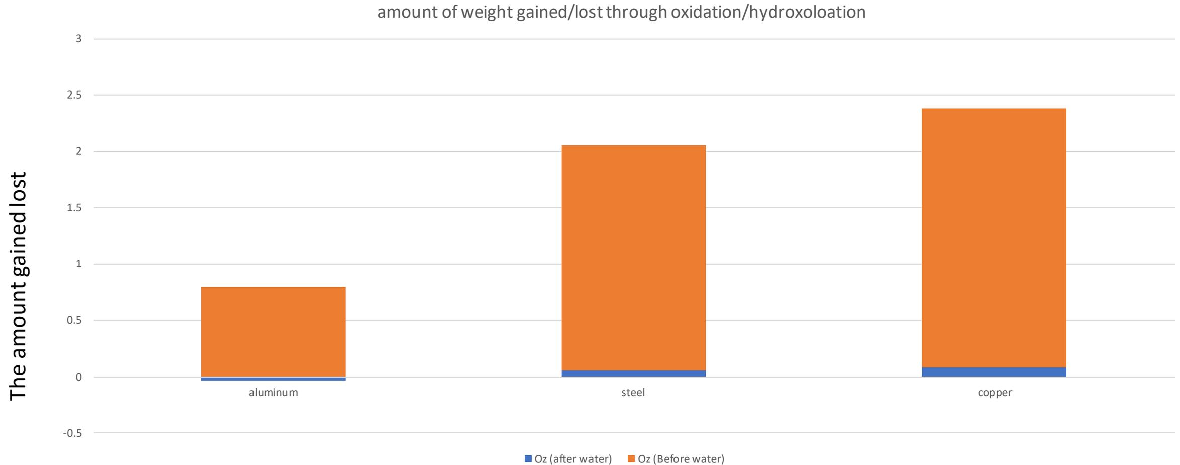
The bar graph will show in a visual form the difference of in weight of the metal in how much it gained or lost (in oz) due to Oxidation/Hydroxylation.
